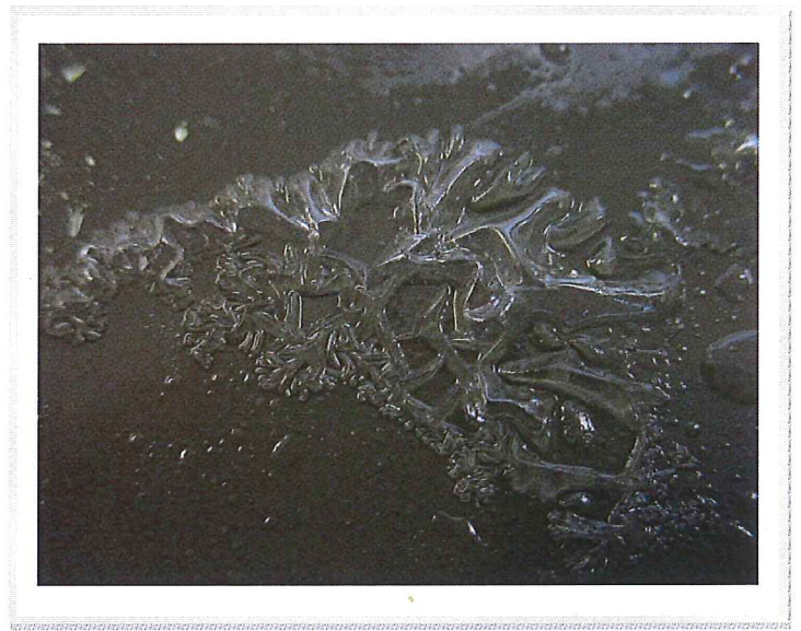
Ronabond EP Cleaner removing 1mm Ronabond EP21SLV film from coated steel panel (40 mins at 23 °C)
